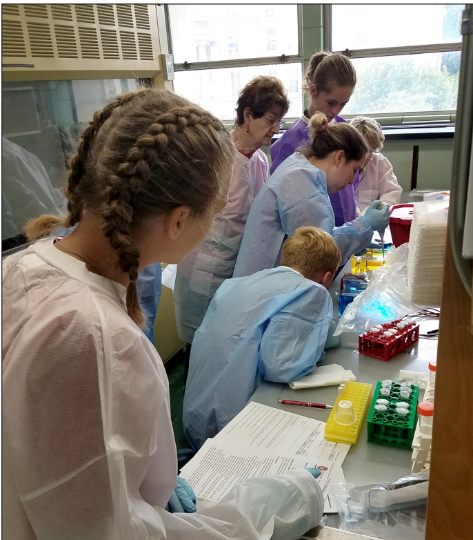
Molecular Geneticist Maureen McCormack demonstrates loading a gel with colored solution. GPU students then loaded their own gels and watched how different molecularly-weighted colored solutions moved through the agarose gel.
