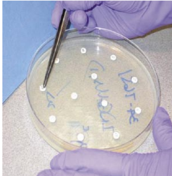
Figure 4.7 —Tapping disks to ensure contact
